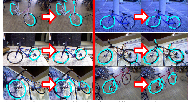
Figure 3. Structure modification from different graph templates (object fragments) to SAPs (fuzziness \tau = 0.4 ).
